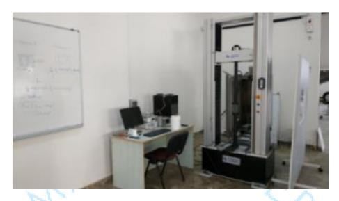
Tensile Test Machine (Mechanical Workshop)
